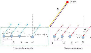
Signal transmission and reception in FDA-MIMO radar.
