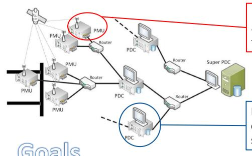
PMU (Phasor Measurement Units), Data acquisition device that uses the GPS system to perform synchronized measurements.
