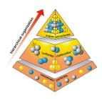
layer of big spheres periodically patterned on the surface of which there is a second layer of spheres, proportionally reduced in size (Polystyrene).
