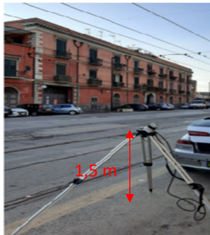
(a) Street-view of the experimental site. (b) Set-up adopted to carry out the experiments
