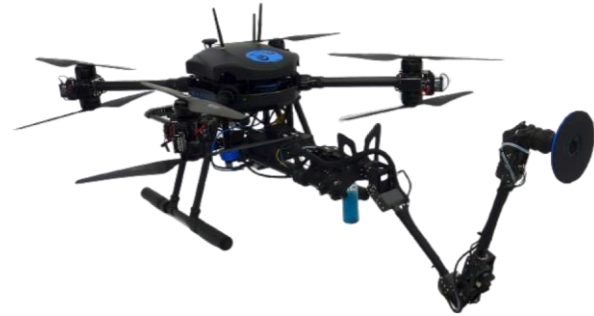
NDT drone: platform developed at PRISMA Lab
