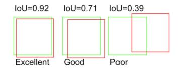
Model's performance was evaluated using different IoU thresholds.
