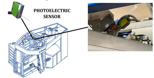
When a Buffalo enters the robot, the **Photoelectric sensors output** switch from: **LOW-SIGNAL** (0 logic)
